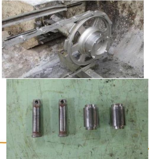
The image shows a sprocket and four bushings for the YK WRP. The sprocket is shown in a close-up view, and the bushings are arranged horizontally below it. They are set against a green background.  |
