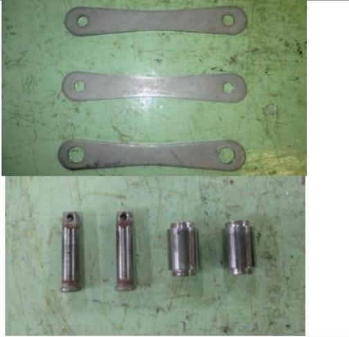
The image shows three metal links and four bushings for the GS WTP. The links are arranged vertically, and the bushings are arranged horizontally below them. They are set against a green background. |
